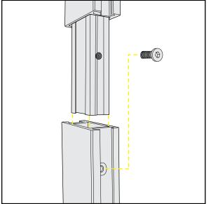
Inline Connection between Extrusions
